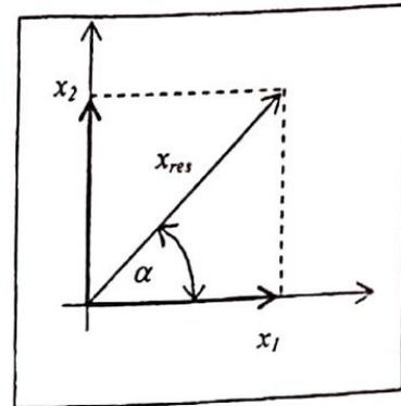
$$x_{res} = \sqrt{(x_1)^2 + (x_2)^2} = 10 \quad ; \quad \text{tg}(\alpha) = \frac{x_2}{x_1} = \frac{8}{6} \rightarrow \alpha = 53,13^\circ = 0,928 \text{ rad}$$
